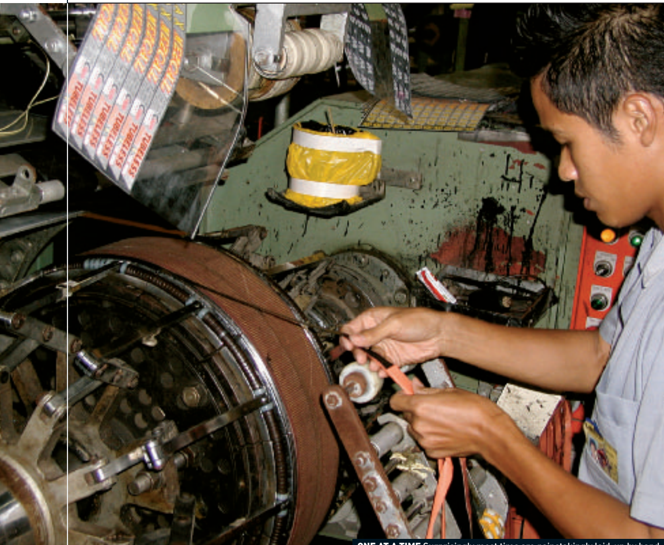
ONE AT A TIME Surprisingly most tires are painstakingly laid-up by hand.
