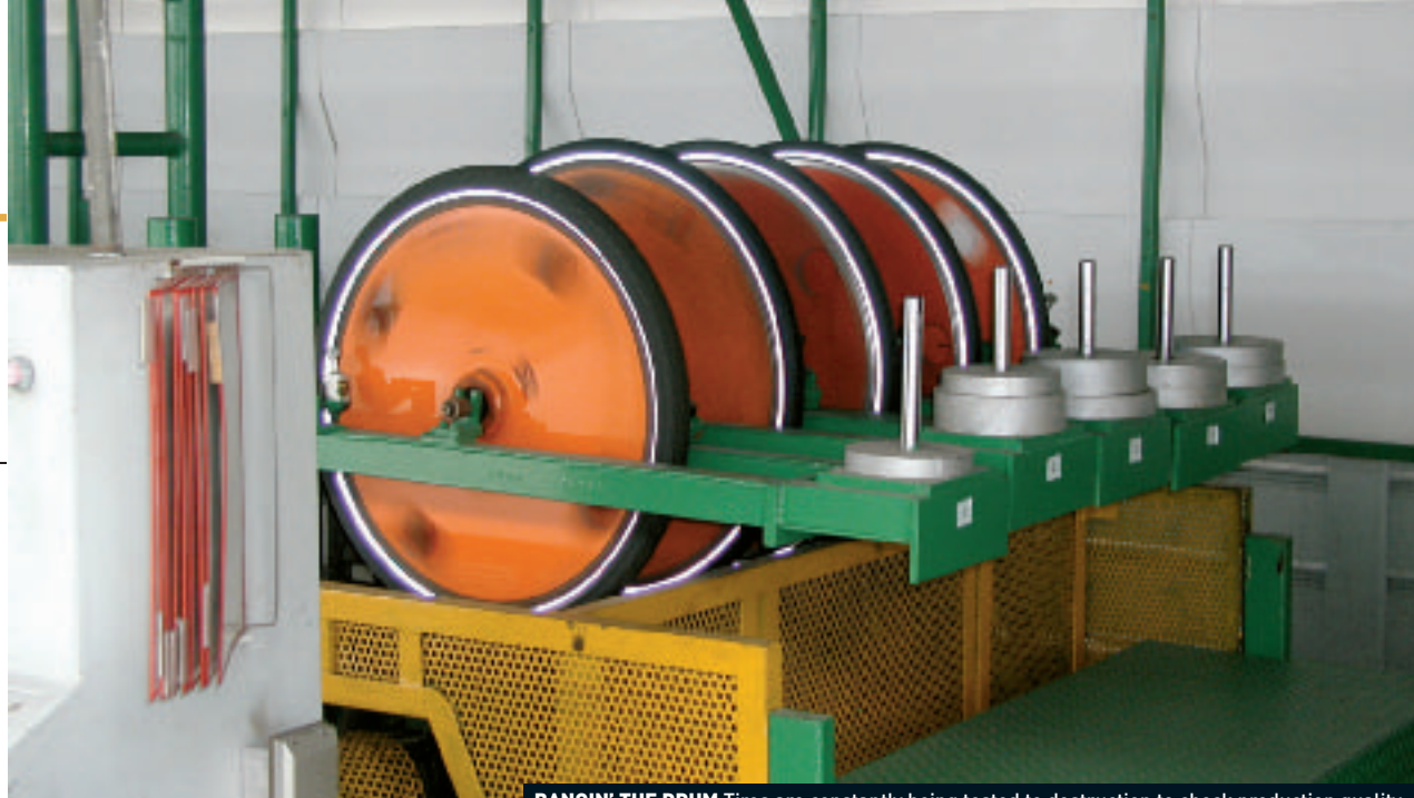
BANGIN' THE DRUM Tires are constantly being tested to destruction to check production quality.
