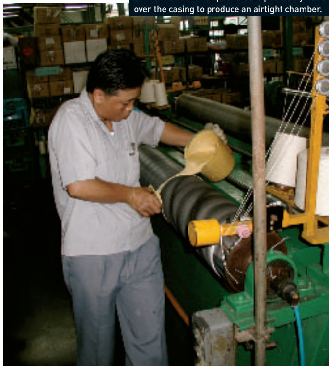
STEADY STREAM Liquid latex is poured by hand over the casing to produce an airtight chamber.
